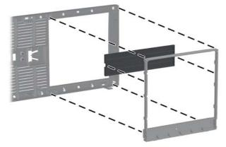
NOTE: When replacing the subpanel, ensure that the aligning pins and any remaining bezel blanks are in their proper orientation. The logo on the subpanel should be located at the bottom of the subpanel when properly oriented.
